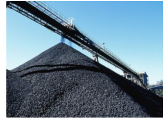
Figure 4.10: The inclination angle of coal piles depends on friction force. If they get wet in a rainfall, they may become dangerous.
