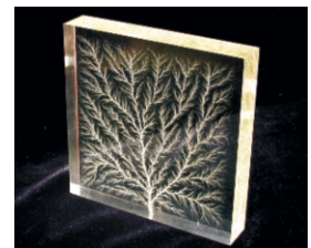
Figure 17.12: Cracks formed on a plexiglass plate as a result of dielectric breakdown.
