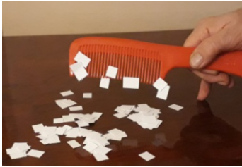
Figure 14.2: A comb rubbed with a piece of cloth attracts small pieces of paper.
