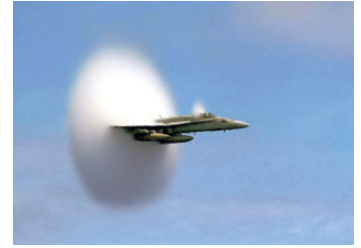
Figure 10.19: The shock wave formed when a fighter plane exceeds the sound barrier causes the air to concentrate where it passes, and a conic wavefront is observed.
