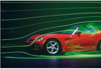
Figure 11.16: Streamlines around an automobile.
