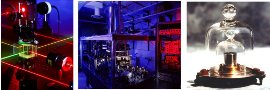
Figure 1.1: The laser assembly that determines the meter unit (left). The cesium atomic clock that provides the second unit (center). The platinum-iridium cylinder stored in France as the kilogram standard (right).
