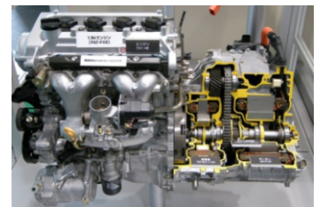
Figure 19.10: Hybrid automobiles have two motors, one gasoline and one electric (right). The electric motor activates at startup and when the speed changes.
