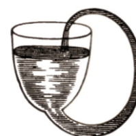
Figure 13.5: The perpetual motion machine suggested by Robert Boyle. In this machine, water will not flow and circulate by itself, because the point at which water exits the hose should be below the surface of the water in the container.
