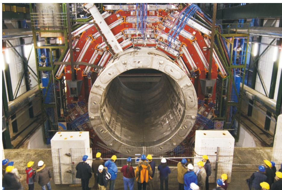
The 2000-ton CMS detector is being inserted into its socket at the CERN European Nuclear Research Center. The superconductor magnet at the center of the detector (the gray area) can generate a magnetic field up to 4 T.
