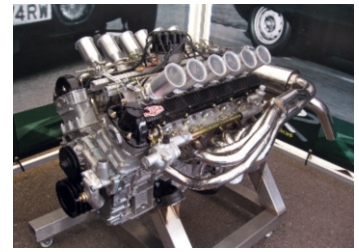
Figure 13.15: The Jaguar V12 engine has a record compression ratio of r=14 .
