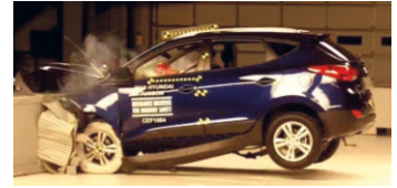
Figure 6.5: Cars are manufactured in such a way that their front and rear parts collapse readily in a collision. Thus, less energy and momentum will be transferred to the passengers.
