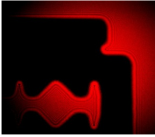
Figure 23.6: Diffraction in the shadow of a razor blade (Lecture Demonstration Services, Harvard Science Center).
