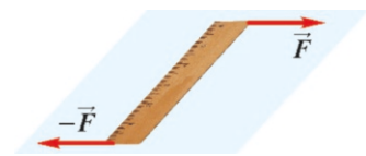
Figure 7.2: The net force acting on this ruler stick is zero. But it is not in equilibrium and will perform rotational motion.
