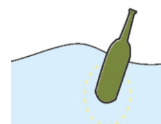
Figure 10.1: A bottle does not move forward as a wave does, it only moves up and down.
