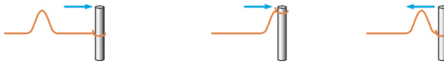
Figure 10.13: A wave reflected from a free end will have the same phase.
