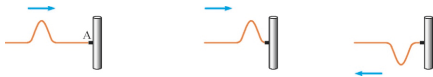
Figure 10.12: A wave reflected from a fixed end will have a 180^\circ opposite phase.
