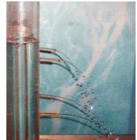
Figure 11.22: Velocities of water at various depths according to Torricelli's formula.
