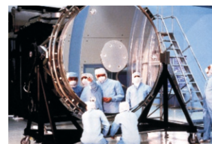
Figure 22.19: The concave mirror used in the Hubble space telescope.
